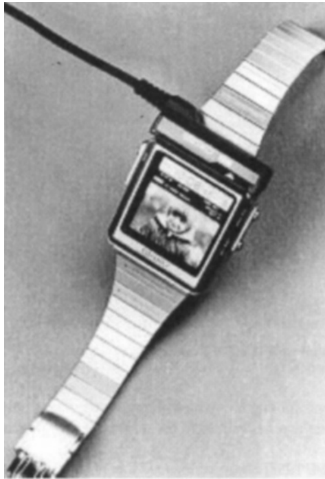
Figure 20.1 Seiko pure crystalline silicon transistor wrist television. From Kawamoto, H. 2002. Proc. IEEE , 90 , 4, 494, April.
