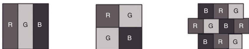
Figure 22.11 Subpixel arrays of the vertical, square, and delta configurations.
