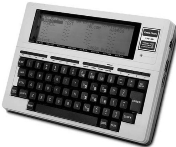
Figure 18.6 Tandy hand-held computer made by Kyocera displaying a full eight rows of text on its liquid crystal display. From http://www.oldcomputers.net , courtesy of S. Stengel.
