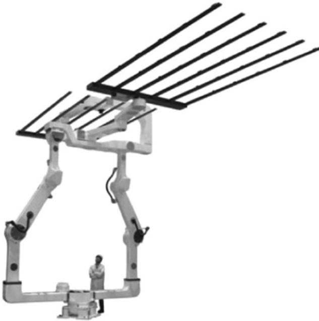
Figure 25.7 Glass panel delivery robot. From yaskawa.co.jp .
