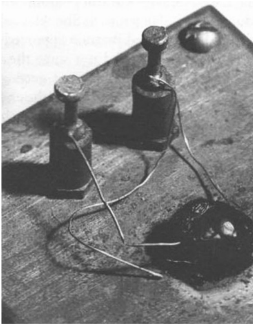
Figure 19.7 Bell Labs photo of Shockley's junction transistor experimental apparatus.
